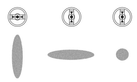
A) Loosen the collar 6094. Turn the air cap 6093 to the horizontal position then re-tighten to collar to lock it into place. This setting produces a vertical spray pattern. This pattern is used more than any other by experienced spray painters.
