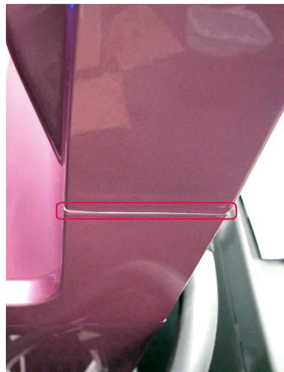
Horizontal edge under the display panel is unpainted.
