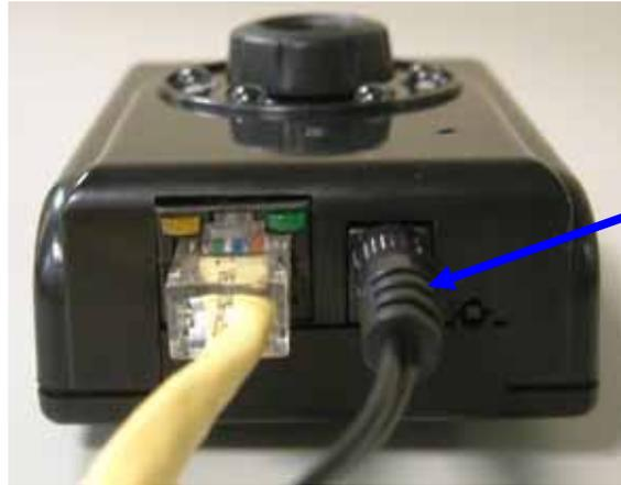
Once you have installed the Network Camera well and powered on, the network accessing type LED will turn green first and then orange. It means the system is booting up successfully. Furthermore, if you have a proper network connection, and access to the Network Camera, the 10/100M LAN LED will flash green
