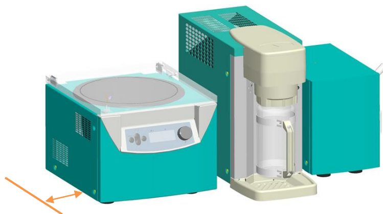
50 mm air gap around system
