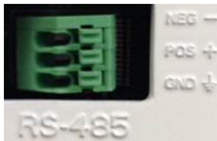
Figure 13: IP Ultra RS-485 Pin-Out (Pin 1: NEG, Pin 2: POS, Pin 3: GND)
