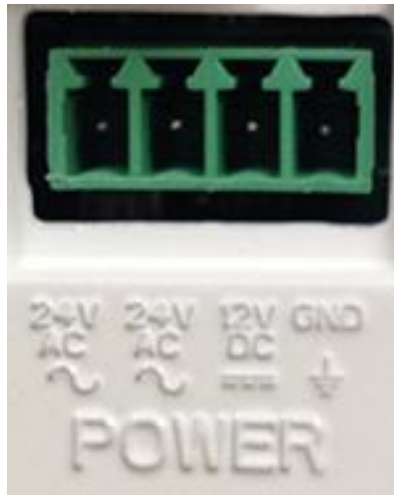
Figure 12: IP Ultra Pin-Out (Pin 1: 24 VAC, Pin 2: 24 VAC, Pin 3: 12-24 VDC, Pin 4: GND)
