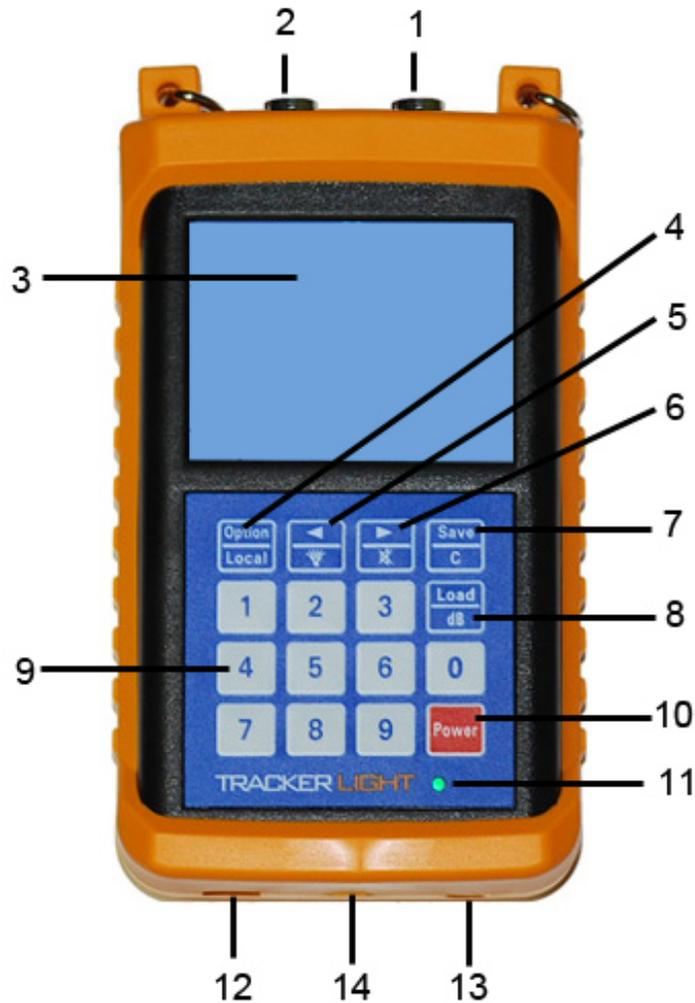
1. Input port: The port to connect with LNB (Satellite Dish LNB)
