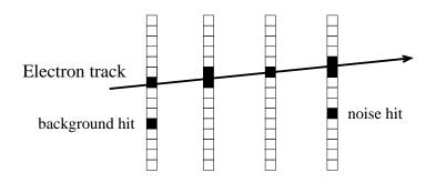
**FIGURE 1.** Illustration of a typical event from the Compton electron detector. Four planes of sensitive strips are shown. For clarity, only 15 strips per plane are shown, while the actual detector will have more (table 3). The electrons passing through will leave hits *if* the strip was efficient. There may also be background hits, e.g. from synchrotron radiation, and noise hits, as illustrated.
