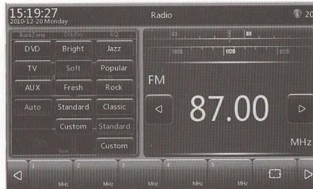
When click time and date area on the upper right screen ., then bring out BackZone、 Display、 EQ fast setup menu.
