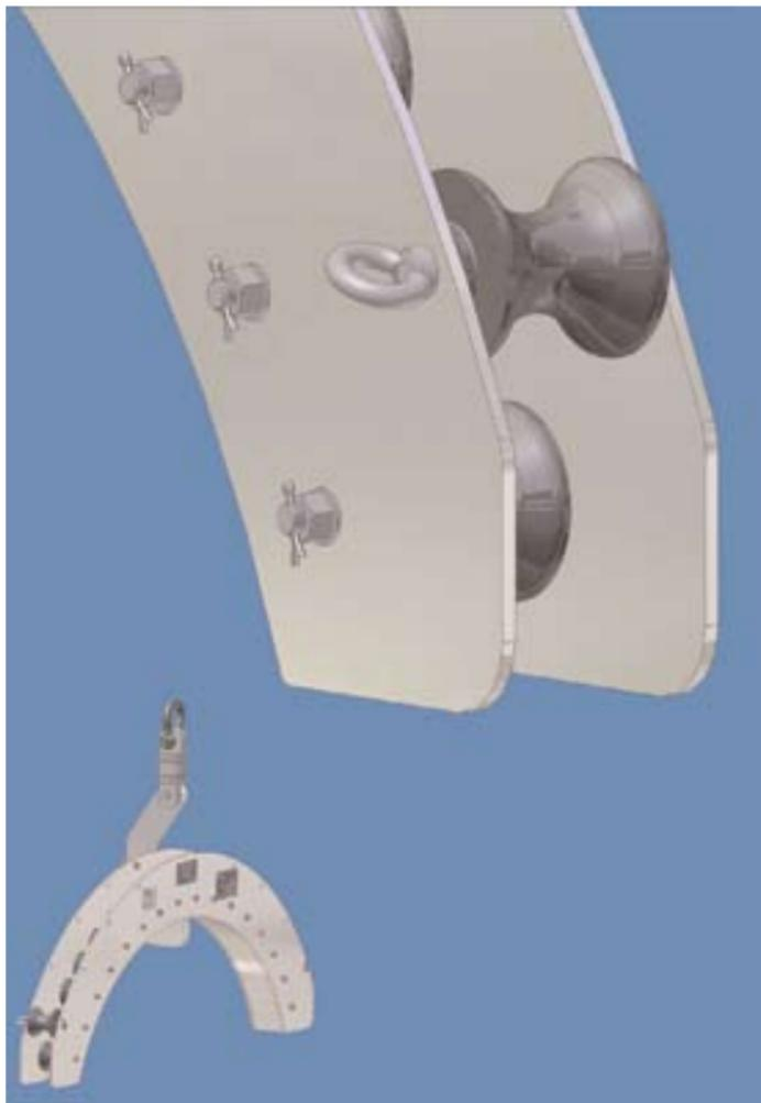
As a result of inadequate securing of rollers in umbilical roller sheaves, there have been several serious incidents where rollers have worked loose and fallen onto the deck.
