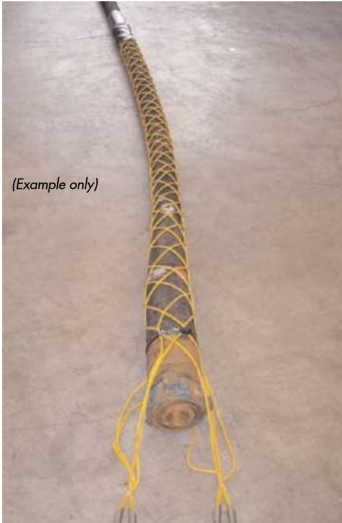
Securing hanging hoses, in particular jet water hoses, presents a safety problem. Use of clips and chains has proven unsatisfactory. With their many parts, the clips themselves constitute a falling object risk. Incorrect positioning of clips and chain loops that are too long have resulted in breakage/bursting and hoses falling down.
