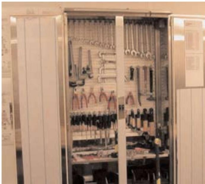
Tool cabinets for work at height are now readily available and employed on many facilities. Unfortunately a number of irregularities have been registered with respect to the way in which the tools are secured and the registration of tools in use and returned tools.
