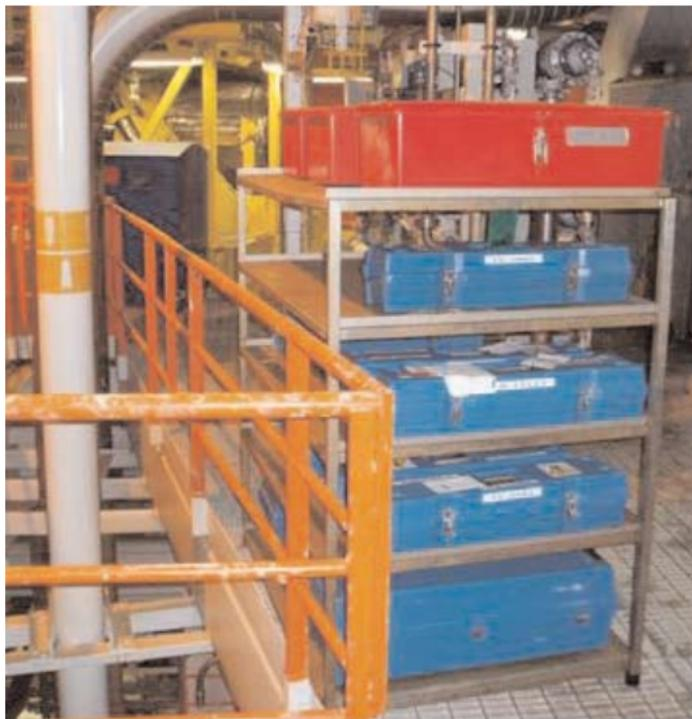
Many cases have been discovered where the design of racks for temporary storage of materials and equipment do not ensure safe storage.
