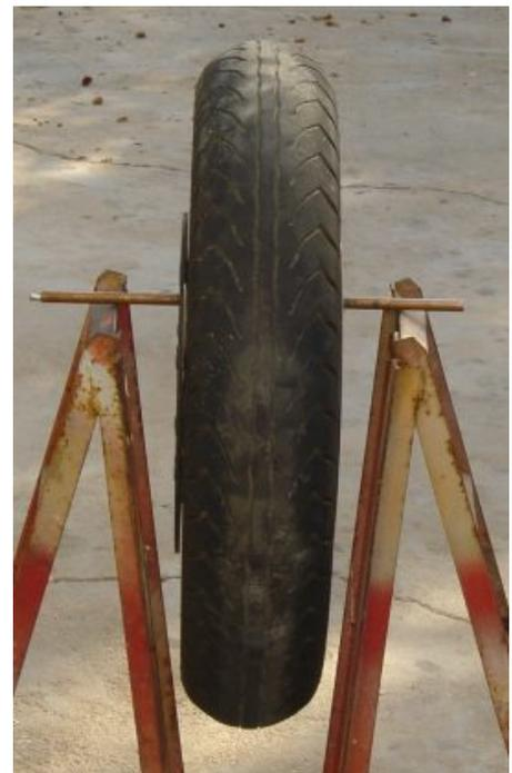
The previous photos show how the wheel needs to be mounted off centre such that it can swing from side to side about an axis defined by the supporting bar. In cases where there is no convenient symmetrical supporting locations (rear wheels and single disc fronts), the wheel can be supported by the bar just under the rim section.
