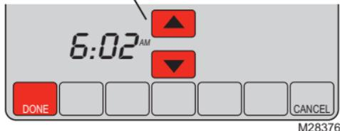
To set the current time display, press **CLOCK**, then press ▲ or ▼ to adjust the time. Press and hold ▲ or ▼ to advance the time more quickly.
