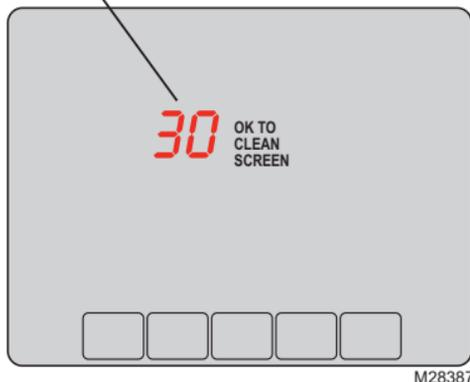
Press **SCREEN** to lock the screen for cleaning. The screen will remain locked for 30 seconds so you can clean the screen without changing any settings.
