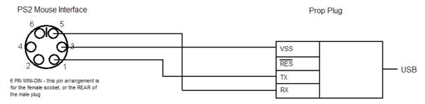
This cable can be used in either a mouse or keyboard port, and is used *in addition* to the normal serial connection to the Propeller via pins 30 and 31. This cable can be used to load *any* program, but is specifically intended to be used to load *XMM* programs, once a suitable loader (i.e. the Mouse Loader) has been loaded via the normal serial connection. After the XMM program has been loaded, the normal keyboard or mouse can be replaced for normal program use.
