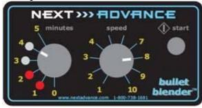
The figure above shows the Bullet Blender<sup>®</sup> set to run for 4 minutes at a speed of 8, after running for 2 minutes. To operate, press the "START" button. After the first minute, the LED light by the number 1 will light up. After the second minute, the second LED light by the number 2 will light up. And so on. At the settings shown above, after 4 minutes, the Bullet Blender<sup>®</sup> will stop. In the Blue versions, the words "Air Cooling<sup>TM</sup>" will light up in blue during
