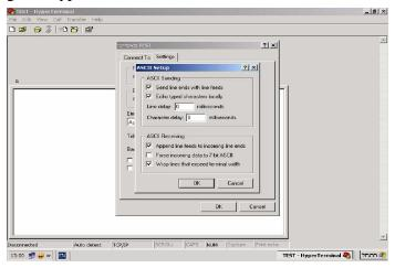
Open the HyperTerminal on 19200 frequency. This Enables you to send AT Commands/Data.
