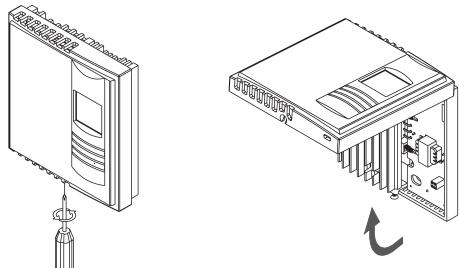
Make the appropriate connections. Please note that the thermostat wires are non-polarized; either wire can be connected to either terminal.
