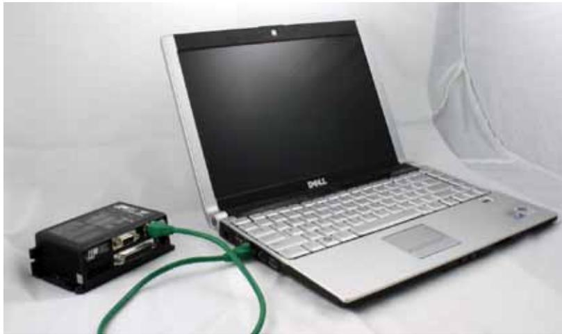
don't need a special "crossover cable"; the drive will automatically detect the direct connection and make the necessary physical layer changes.
