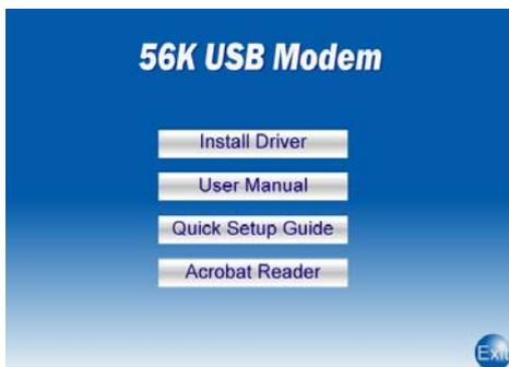
3. A ” **Install Driver**” window will pop-up. Click “**Windows 2000&XP**” and Window system will automatically install the driver!.
