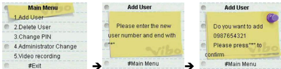
In main menu, press 1 key to enter new user adding interface. Enter the phone number of the new user, and end by pressing “\*\*” key. Press “\*\*” key again to confirm the operation, press “#” key to cancel the operation and go back to main menu.
