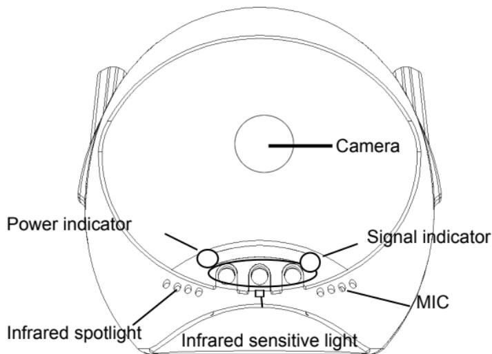
**Camera:** It can rotate upward at an angle of about 40 degrees, downward at an angle of about 5 degrees, and left and right at an angle of about 45 degrees.
