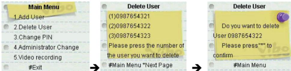
In main menu, press 2 key to enter user deleting interface. Press “\*” key for paging down. Select the serial number before the phone number you want to delete. Press “\*” key to confirm the deleting, press “#” key to cancel the operation and go back to main menu.
