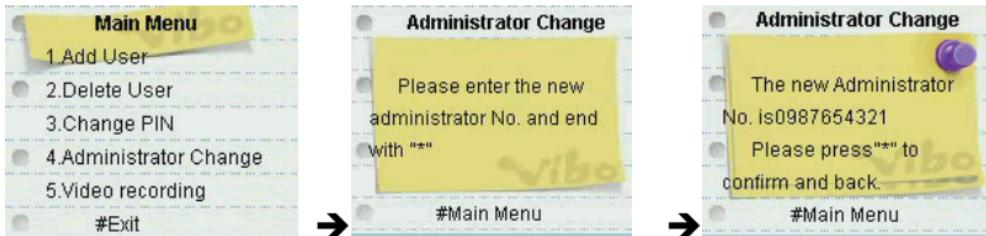
In main menu, press 4 key to enter AD number interface. Enter the new AD phone number (EX: 09\*\*\*\*\*) and end by “\*\*” key. Press “#” key to cancel operation and go back to main menu .
