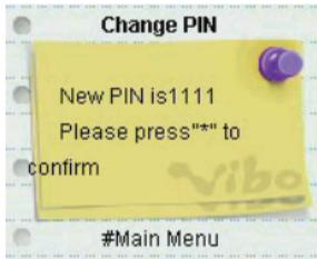
In main menu, press 3 key to enter password editing interface. Enter the current password and end with “\*” key, then enter the new code and end with “\*” key. Press “\*” key to confirm the input.
