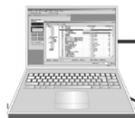
FRENIC loader Allows operation of the inverter connected on-line with the PC.
