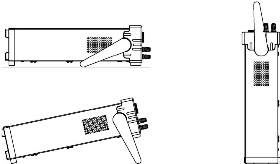
Diagram 3.3 YI-55 Series Power Supply Viewing Positions
