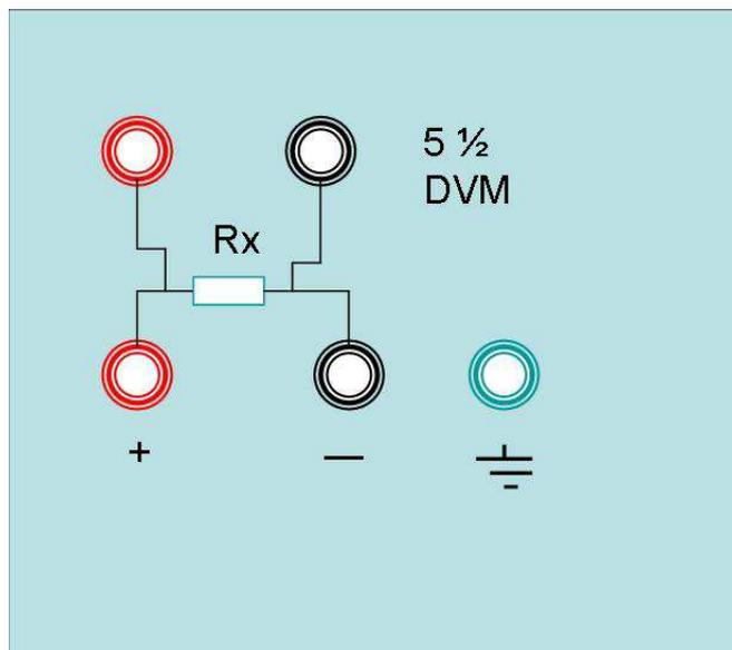
Diagram 4.5 Milliohmeter Measuring Resistance
