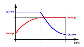
In "Current generator" mode, it's possible to connect any type of battery or other loads to the charger. The output current is regulated from zero to the maximum value with the appropriate potentiometer and the timer is used to set the total time of charger (at constant current). This feature is useful to recover old sulphated batteries or to charge stacks of cells.
