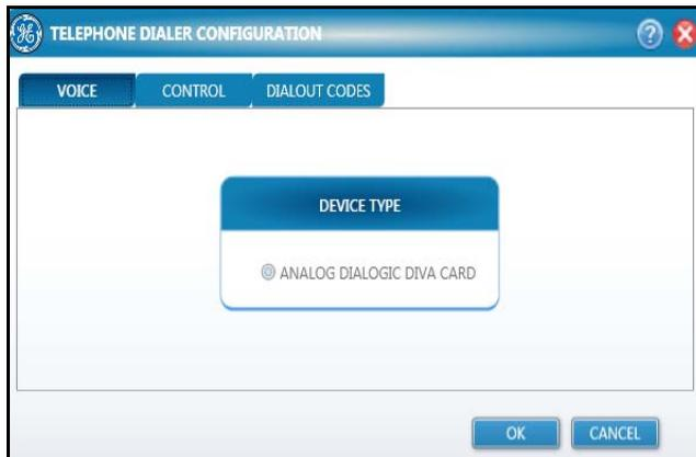
Figure 88: Voice Tab in Telephone Dialer Configuration
