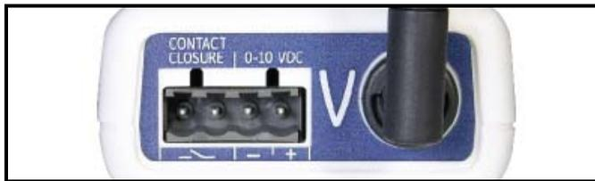
Figure 10: Auxiliary Input Terminal
