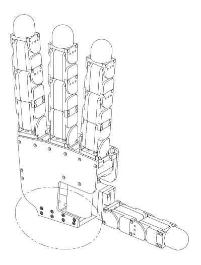
Remove six (6) screws on either side of the hand.
