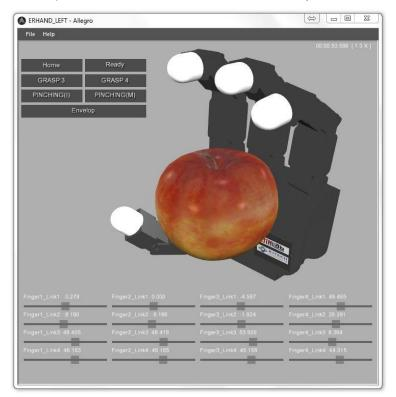
AHAS is provided along with the Allegro Hand for two main purposes. AHAS allows for ease of testing CAN communication between your PC and the Allegro Hand hardware. Secondly, AHAS provides several robust grasping algorithms for use with the Allegro Hand. The algorithms provided with AHAS can grasp a variety of object geometries for demonstration or for use at the end of a manipulator.
