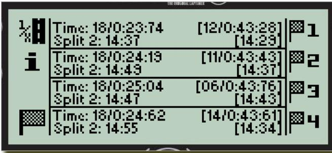
The screenshot shows a digital display with four rows of data, each representing a driver. Each row contains a driver icon, a current lap time, a best lap time in brackets, a split number, a split time, and a best split time in brackets. The data is as follows:
