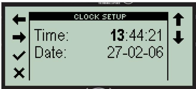
UniWatch includes a real-time clock running even when UniWatch is off.
