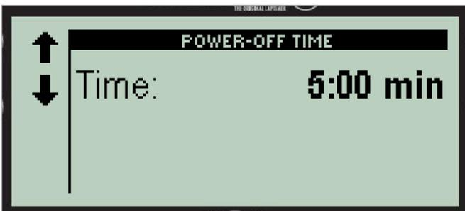
UniWatch will automatically turn itself off if it is not used. To save batteries, you want it to turn off as fast as possible, but on the other hand it should not affect the daily work.
