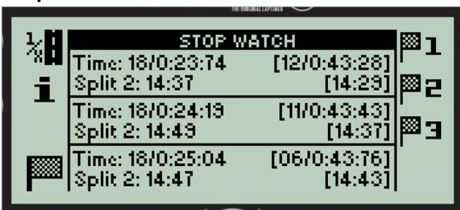
The display shows for each driver the current lap time, the current lap number, the best lap time, the best lap number, the split number, the split time and the best split time.
