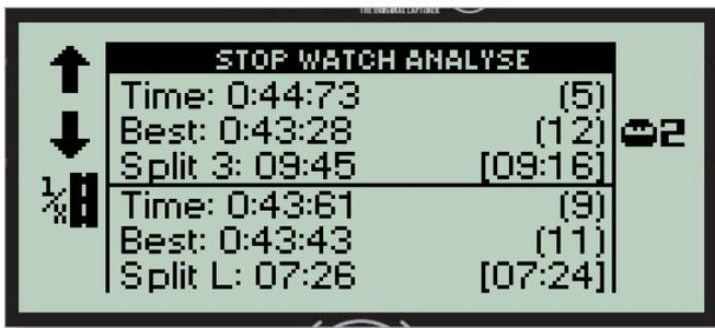
You can adjust the drivers lap number or split number by pressing **and** holding down the driver's button. When you do that, you will see the buttons change and you will now be able to scroll through the laps by using the arrow buttons and toggle through the splits with the split button.
