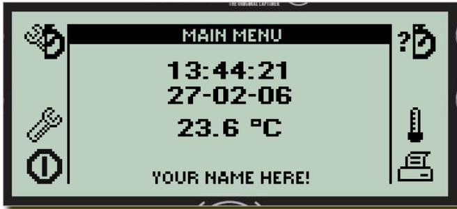
From the main menu you can go to the different menus or turn UniWatch off. On the screen you will see the current time and date and the environment temperature. The environment temperature is measured inside UniWatch and sometimes you will see a higher temperature because you are warming the box with your hands.
