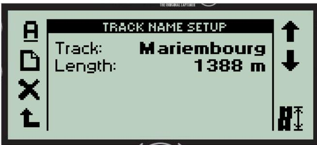
When you press **and** hold the track setup button to the left, you will see the display change. From this new screen you will be able to choose the right track using the arrow buttons to the right. When you have chosen the right track, you release the track setup button again and the track is selected. Just for information, the track
