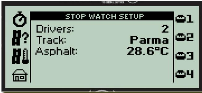
When UniWatch is turned on, it will start in the “Stop watch” setup menu. This is where you set the information relevant for the race before it starts.
