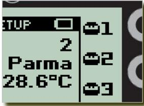
When it is time to change the batteries a small battery symbol is shown in the menu line. This does not mean that the UniWatch will stop functioning. The first sign of really low battery voltage is when the real-time clock is corrupted. The battery icon is shown when the battery voltage is around 2.0V.
