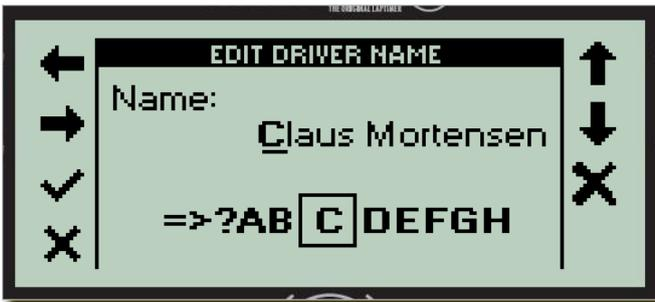
This example is showing the editing of a drivers name. You can move the cursor with the left and right buttons and change the value with the up and down arrow. At the bottom you are seeing the font used for the text. The character in the rectangle is the current selected one from the text. You can see what 5 characters are before
