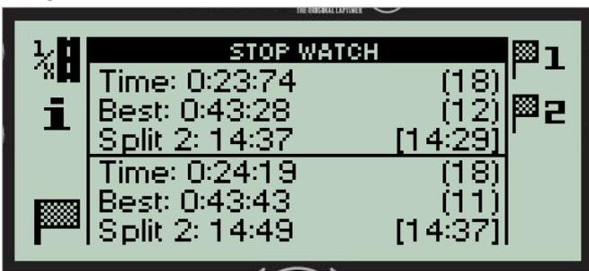
The display shows the current lap time, the current lap number, the best lap time, the best lap number, the split number, the split time and the best split time. Everything is shown for each driver. You can change the driver shown by pressing the driver number.
