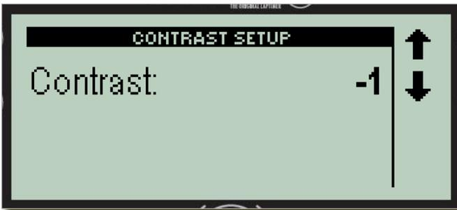
The contrast of the display is the light difference between the dots that are turned on and dots that are turned off. You can manually adjust the contrast setting by pressing **and** holding down the contrast button and then use the arrow buttons. You will see the contrast change at the same time.
