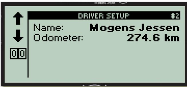
Perhaps you noticed the display changed when pressing the buttons to the right? This is because the buttons have two functions. If you press the button with a short press you chose the number of drivers, but if you press **and** hold the button down, you will set the name of that driver. When pressing and holding the
