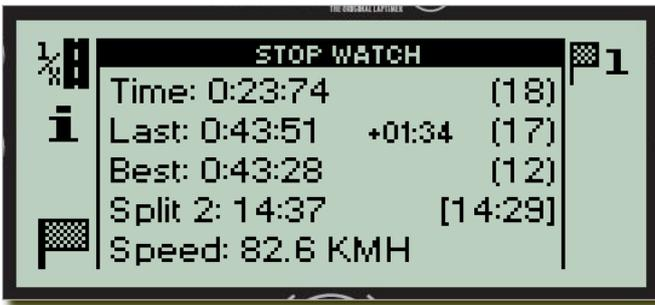
As seen on the example to the left, you have a lot of information in the display. The lap time is the current running lap time. It is showing the running time of the current lap. You can see the current lap number to right, next to the lap time. The last lap time is shown on the line below.
