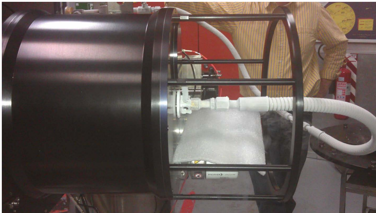
Figure 15: Fill fitting and nitrogen line attached to dewar.
