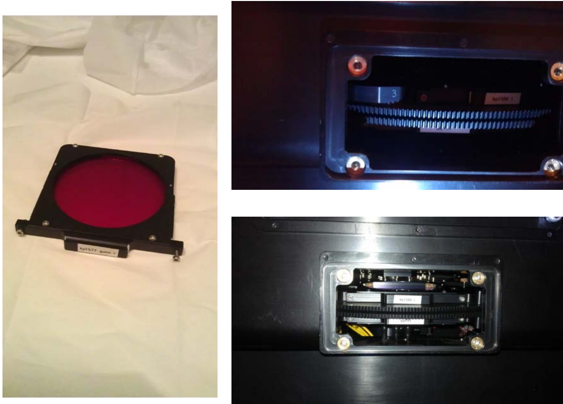
Figure 23: Filter in holder (left), filter installed in wheel, partially rotated to show position number scribed on the wheel (top, right) and different view showing filters installed in both wheels (bottom, right).
