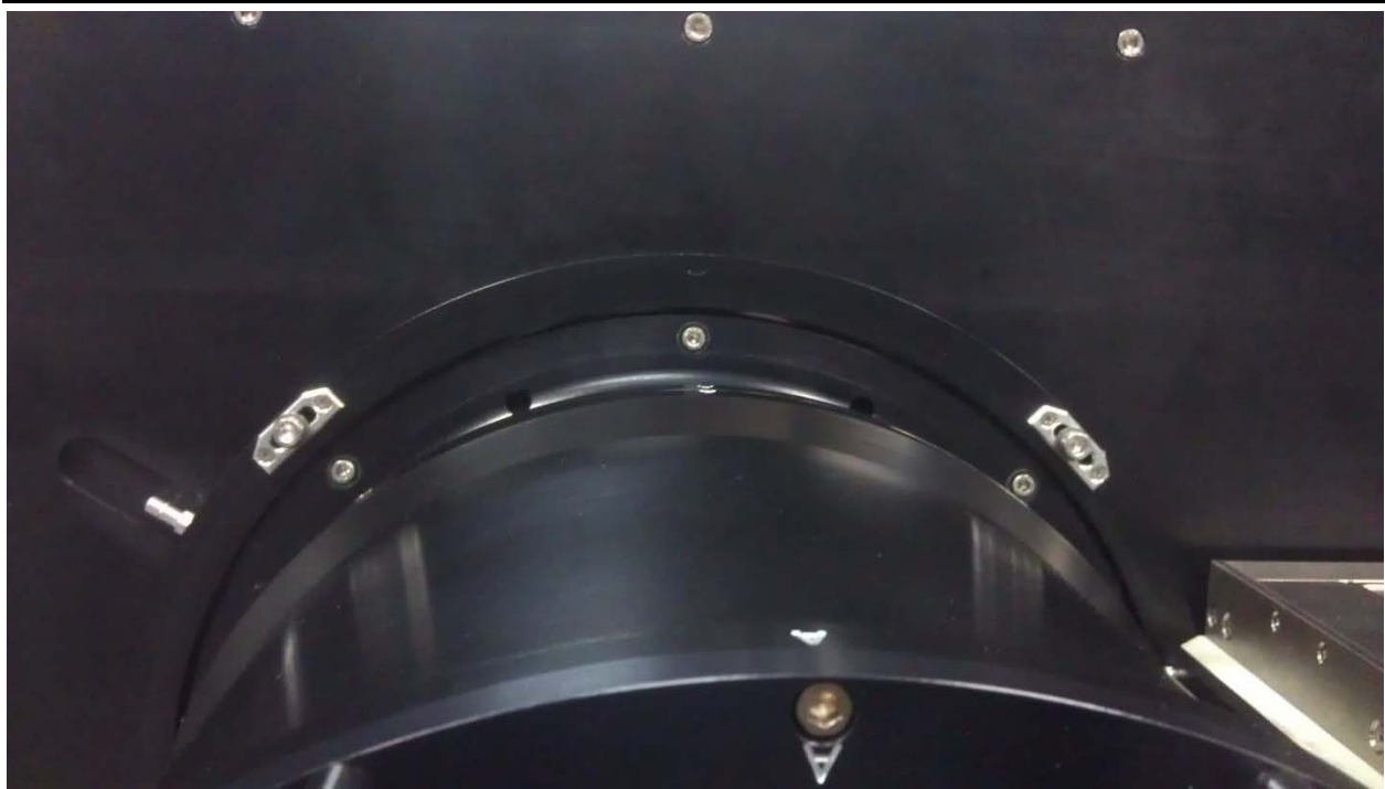
Figure 17: View of COSMOS dewar showing additional slotted attachment points. There are a total of 5. See Figure 10 for KOSMOS features; it has 4 bolts that must be loosened for rotational adjustment
