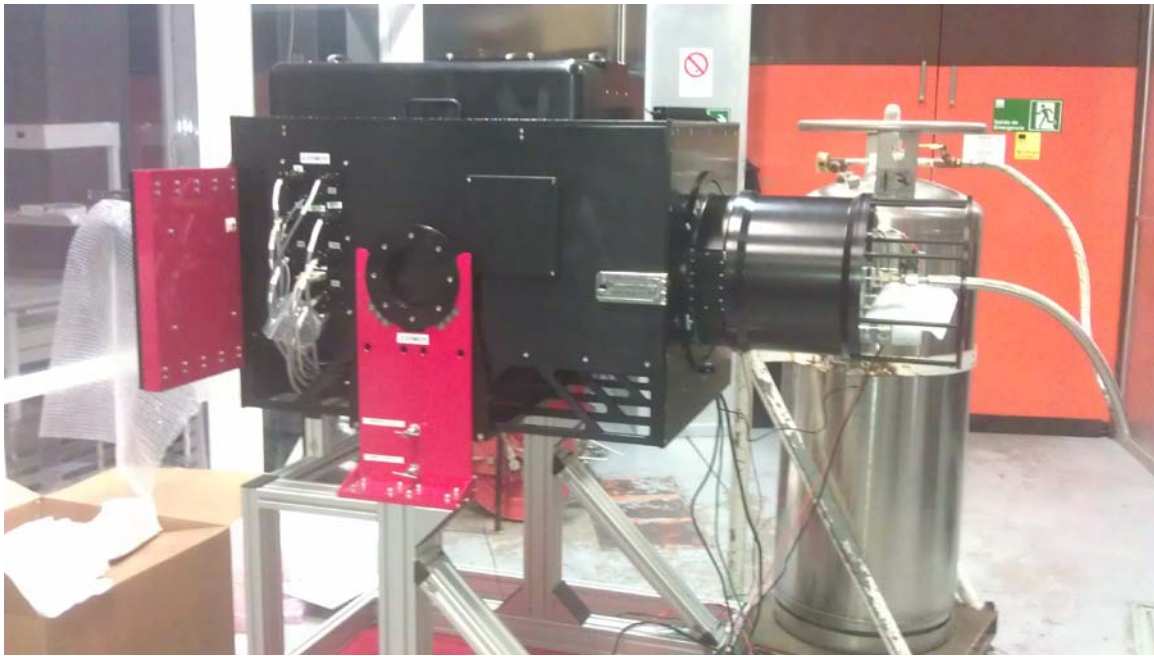
Figure 3: COSMOS on handling cart; note the different dewar design. This figure shows the instrument in the horizontal position with the adapter plate removed.
