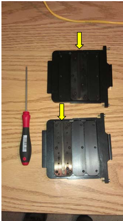
Figure 22: Longslits in holders (left) with ball driver used for installation. The slit holders shown are for a centered slit (top) and a blue-displaced slit (bottom), marked by the arrows. The red-displaced slits have the slit in the position near the handle of the holder. Slit mask mounted in wheel (top).
