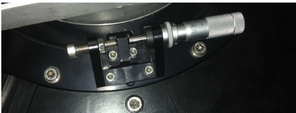
Figure 11: KOSMOS dewar rotation adjustment micrometer. The micrometer for COSMOS is essentially the same.
