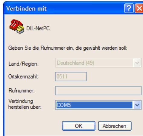
**Figure 5: Direct connection setup with HyperTerminal**
