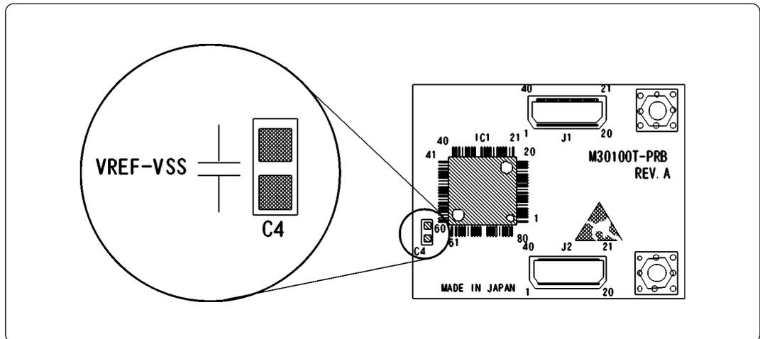
Figure 3.2 Foot patterns of A-D and D-A conversion bypass capacitors
