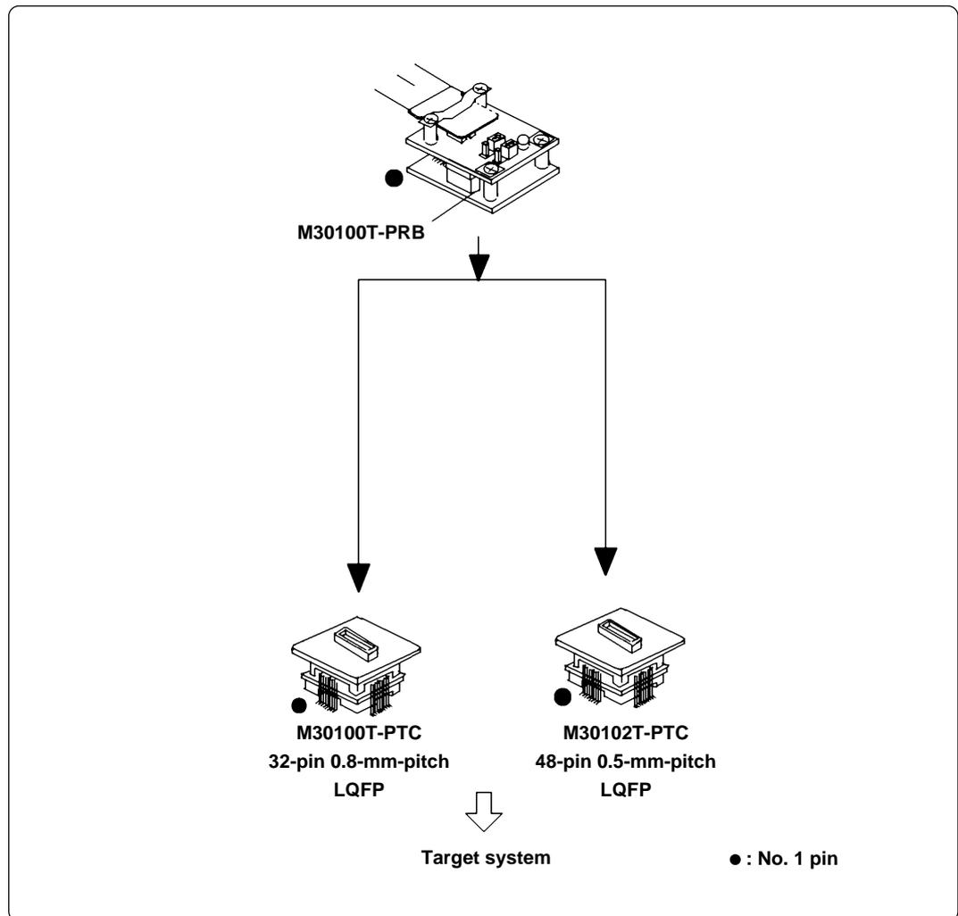
Figure 3.5 Connecting the target system
