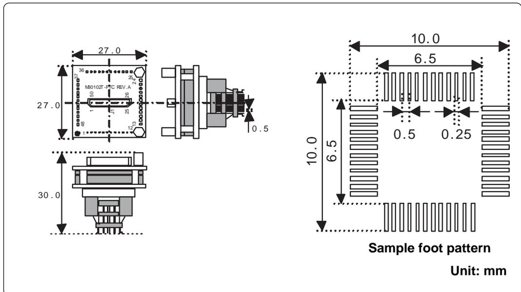
Figure 4.3 External dimensions of the M30102T-PTC
