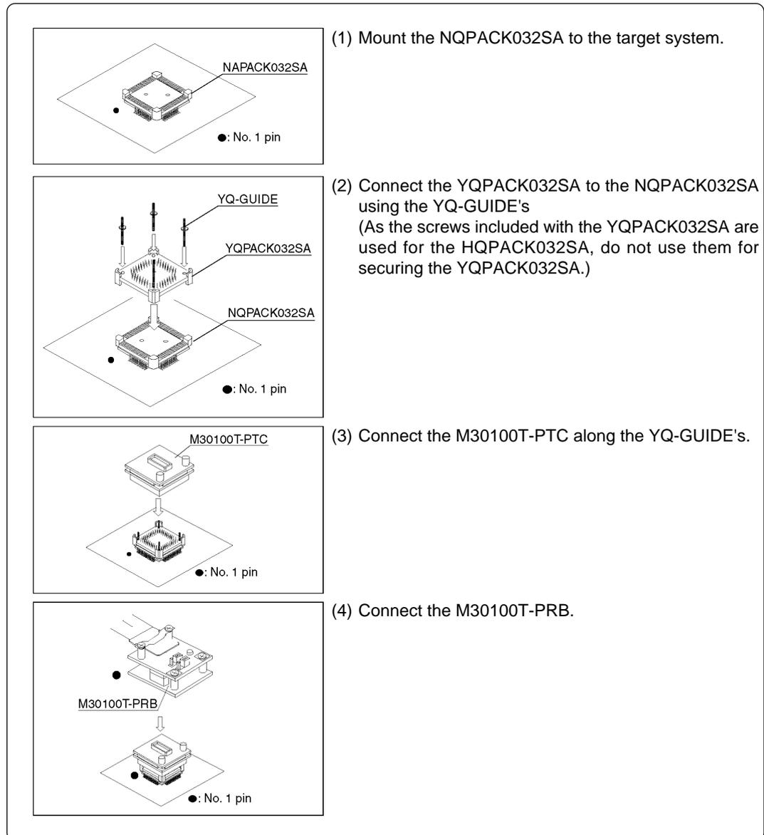
Figure 3.6 Connecting converter board M30100T-PTC for 32-pin 0.8-mm-pitch LQFP
