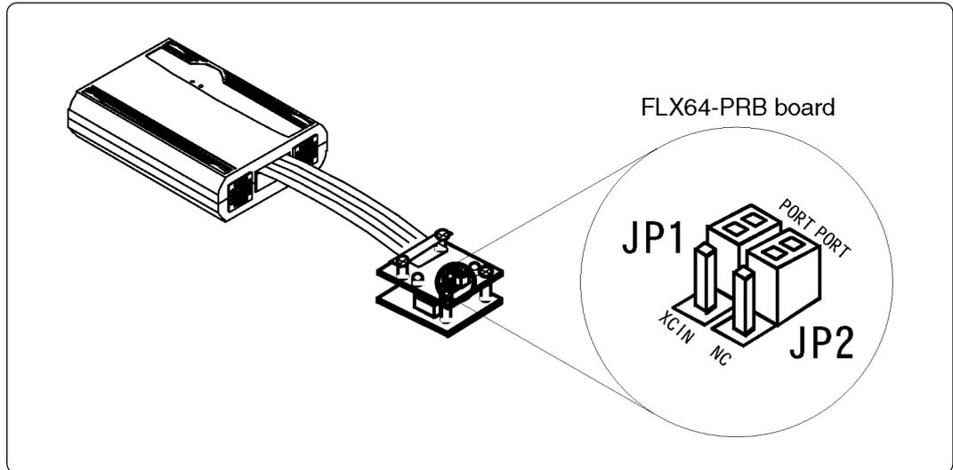
Figure 3.1 Positions of the switches and their factory-settings
