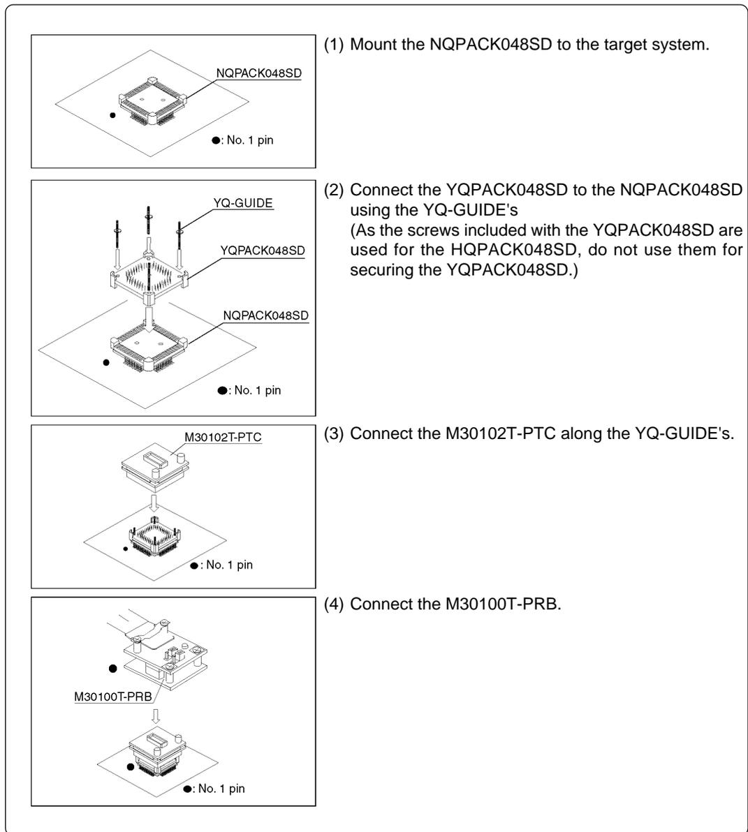
Figure 3.7 Connecting converter board M30102T-PTC for 48-pin 0.5-mm-pitch LQFP
