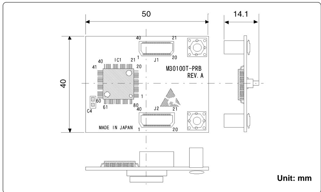
Figure 4.1 External dimensions of the M30100T-PRB
