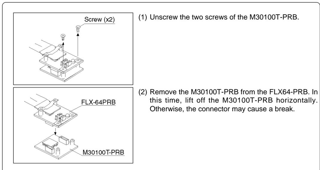
Figure 3.4 Removing pod probe M30100T-PRB
