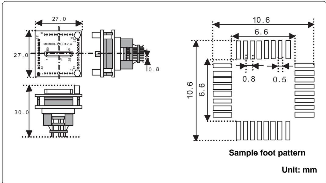
Figure 4.2 External dimensions of the M30100T-PTC
