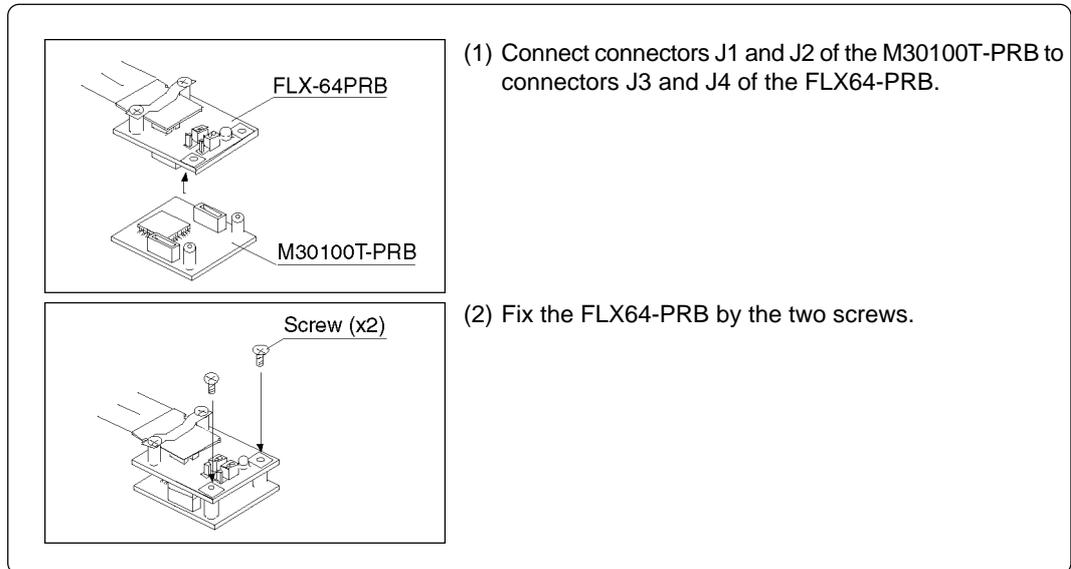
Figure 3.3 Connecting pod probe M30100T-PRB
