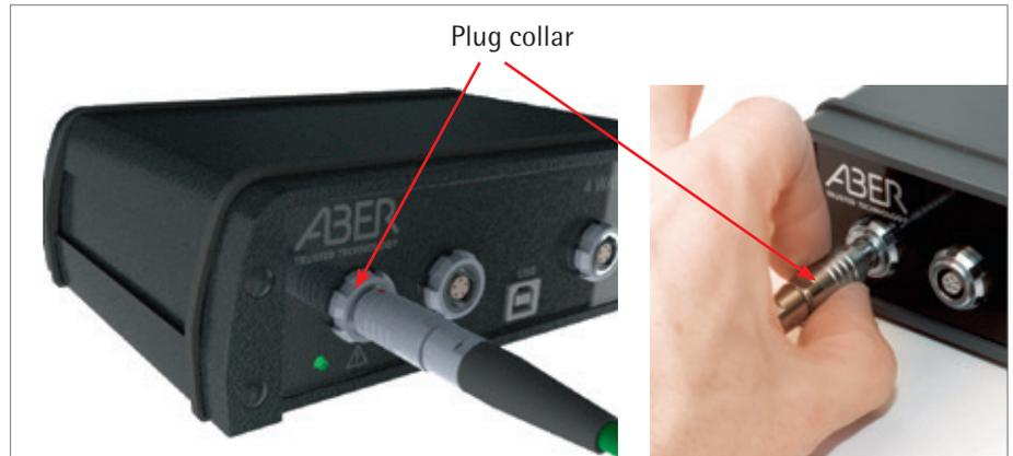
The plug collar indicated must be pulled out a short distance (the distance is almost imperceptible; less than 1mm) from the socket to disengage the lock. Continue to pull on the plug collar to uncouple the plug from the socket. For a cable, hold the collar as shown and pull away from the socket.
