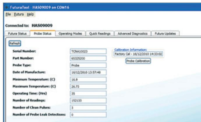
The "Probe Status" tab is very similar to the Futura Status but looks at information taken from the probe instead. The only extra information shown is the number of probe leak detections and calibration details.
