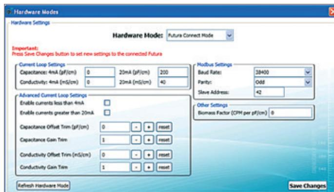
To use Current Loops, enter the capacitance and conductivity values that will correspond to currents of 4 mA and 20 mA in the Current Loop Settings area. The current through the Current Loop outputs will then vary linearly in proportion to the measured capacitance and conductivity values.
