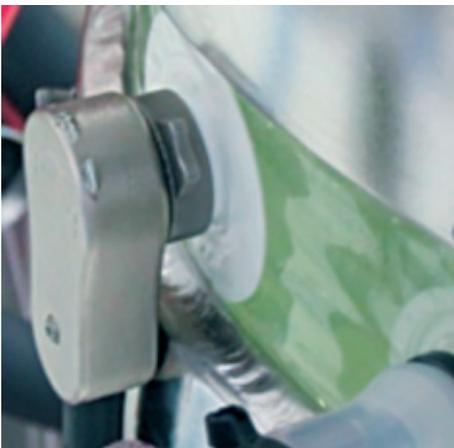
BioPAT® ViaMass comprises of a primary RFI shielded copolymer enclosure for the main electronics and a second copolymer enclosure for the probe connector on a 1 m umbilical cable, both enclosures being RFI shielded and rated to IP41. The 'front end' probe connector enclosure is a lightweight design to minimize stress on the probe and bag.
