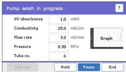
If required, the **Pump wash B** run can be ended before it is completed by tapping **End** to stop the wash in advance.
