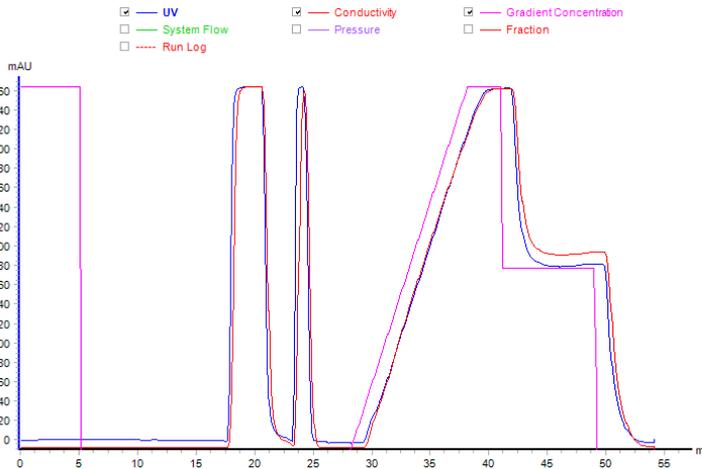
**Note:** It is recommended to optimize the timing of switch valve when wavy gradients or fluctuations are observed. For detailed description, see [Section 5.4.4 Switch valve timing, on page 117](#).
