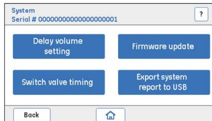
**Result:** Two files with the names INSTLOG.TXT and ERRORLOG.TXT are exported to the USB memory stick.
