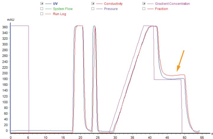
**Note:** Alternatively a manual run of 50% B for 10 min can also be performed to evaluate the gradient fluctuations/wavy gradients.
