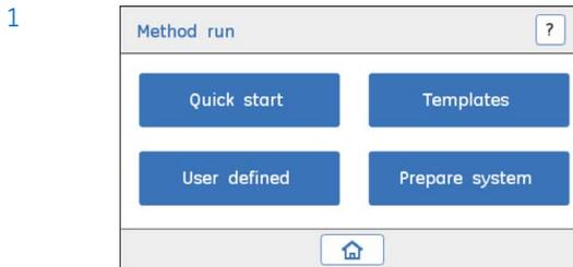
In the **Method run** screen, tap **Quick start** to access the templates.
