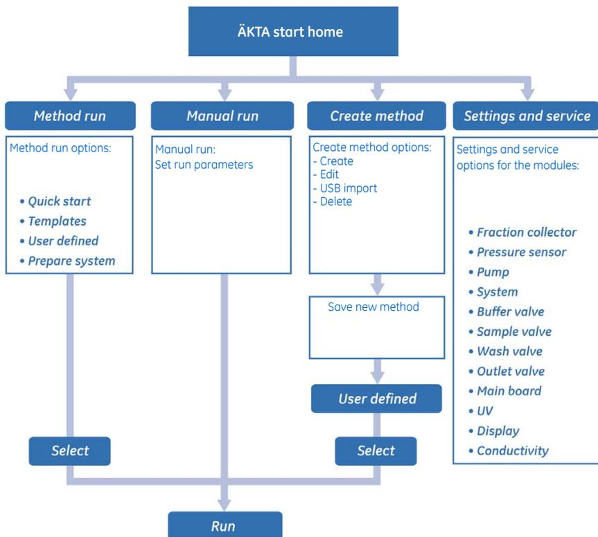
Procedures required after a run, such as the cleaning of the column, the system flow path, can also be performed manually or using methods available in the **Prepare system** menu.
