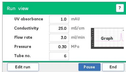
In the **Run view** screen, the following options are available to monitor and control the ongoing run (for details, see [Section 6.3.2 Monitor and control the run, on page 165](#)):
