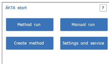
In the **ÄKTA start** home screen, tap **Method run** to access the method types available with the instrument.
