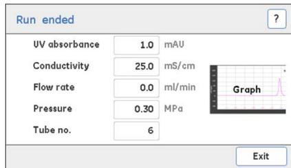
Tap **Exit** to close the **System cleaning** screen when the **System cleaning** run is completed.
