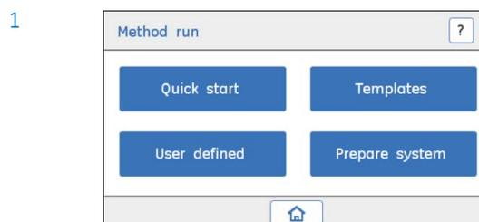
In the **Method run** screen, tap **Prepare system** to access the system methods.
