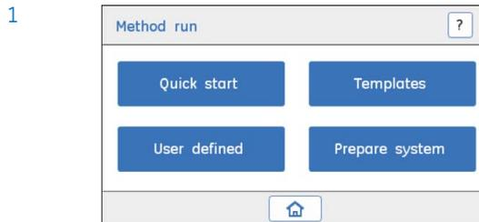
In the **Method run** screen, tap **Templates** to access the different templates.
