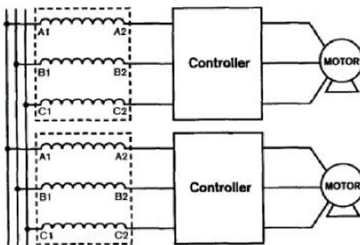
Conventional Line side reactor to VFD connections
