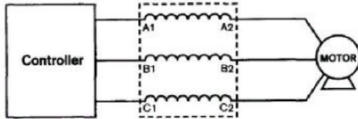
Load reactor connections
