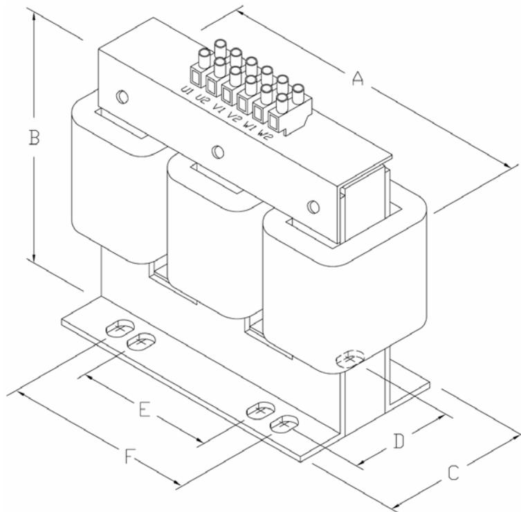
Figure 3 Standard Mounting
