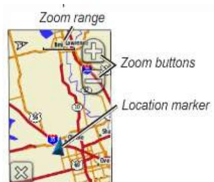
Your current location is indicated by the blue arrow; the head is pointing in the direction, or course, you are currently traveling. To display a different location on the map, touch the map and drag your finger across the display to move the map. Touching the return arrow at the bottom left hand corner of the map will return the map to be centered about your current location.
