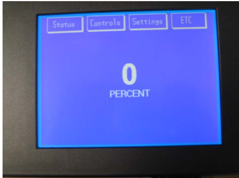
Figure 5 – Numeric Bladder Volume Display
