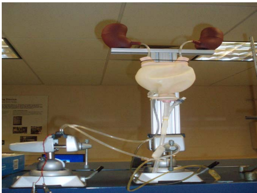
Figure 24 - Inflatable Cuff and Micro-Pump Setup
