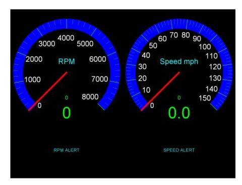
**Dashboard** – Selecting Dashboard will display the two gauges selected in the *Dashboard Settings* panel as shown on page 9. This display is a full screen display and makes it easy for the driver to monitor the chosen parameters without having to focus on the smaller gauges on the *Data Display* screen. If the preset alert values are reached, a colored box will appear next to the respective alert text.
