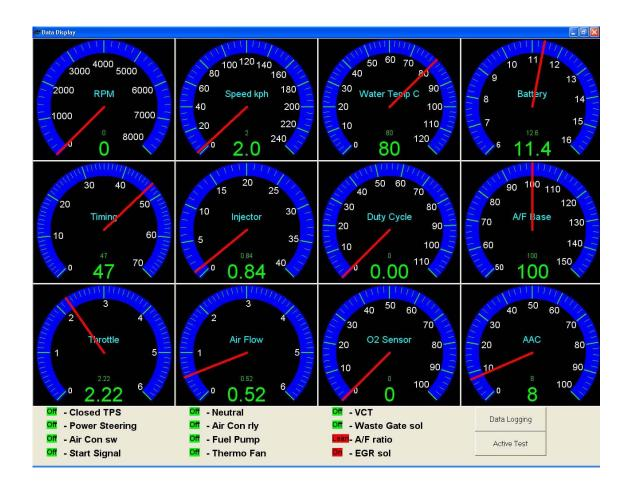
**Data Display** – After configuring the *Data Display* options in the *Settings Menu*, selecting the *Data Display Function* will bring up a display of all the gauges that were assigned a function. These gauges display actual data as provided to the ECU in real time.
