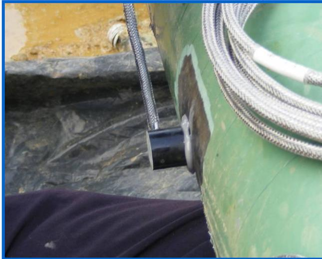
Figure 4.8 – After locating the best spot for mounting with the epoxy.
