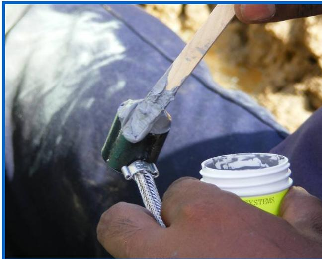
Figure 4.7 – Epoxy Applied to the Face of the Transducer.
