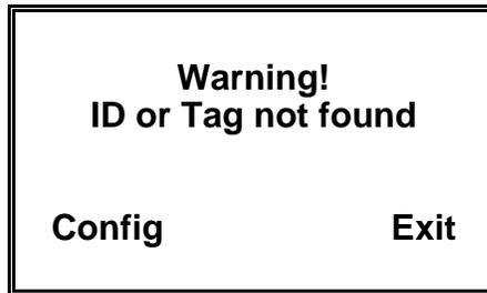
Press **Config (F1)** at this time to manually configure a probe if desired. Follow the instructions on **Manually Configure Probe and Save Setting to the Ultracorr**.
