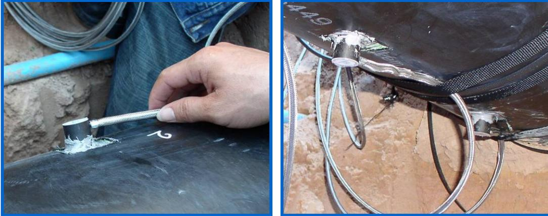
Figure 4.6 – Transducers Being Mounted on Pipeline.
