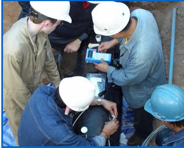
Figure 4.5 – Finding the Location of Lowest db Reading.
