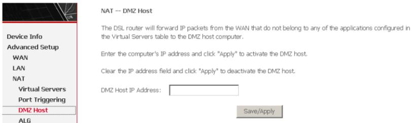
Figure 3 DMZ host configuration
