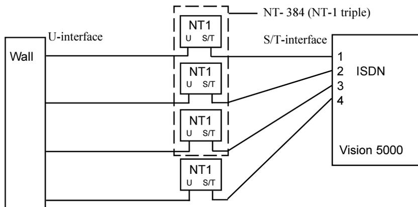
Connect the U-interface of your NT1 adapter to the line provided from your network provider.
