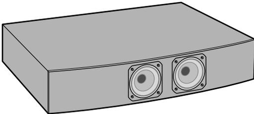
The Natural Audio module is designed to improve audio quality during a videoconference. It is mounted in the cart above the Codec and consists of an audio system optimized for speech. The monitor speaker is not used when using the Natural Audio module. See ‘Peripheral Equipment’ for further information.
