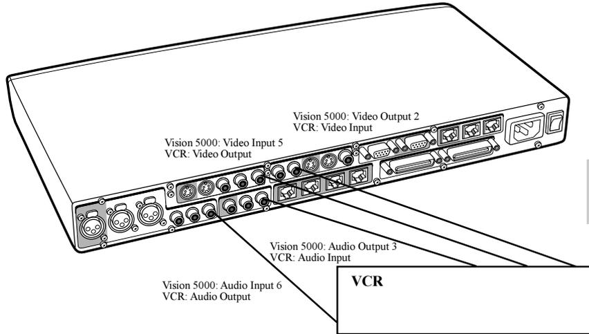
To simplify connecting a VCR, the necessary connectors are marked 'VCR'
