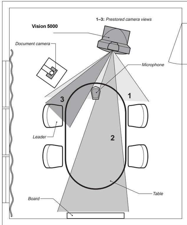
The microphone should be placed at the front of the table to ensure that all speech will be detected. The best position for the microphone is at least 2 meters (6.5 feet) in front of the Vision 5000 on a plain, flat table with at least 0.3 meters (12 inches) of table in front of the microphone.
