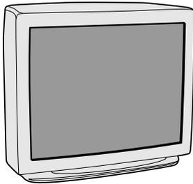
The monitor displays the far-end and near-end videoconferencing sites. The standard system also utilizes the built-in speaker of the monitor. If the Natural Audio module is installed (optional), the monitor speaker is not used. The monitor is also used for displaying the Vision 5000 menus, on-screen help, video from connected video sources and high-resolution still images.
