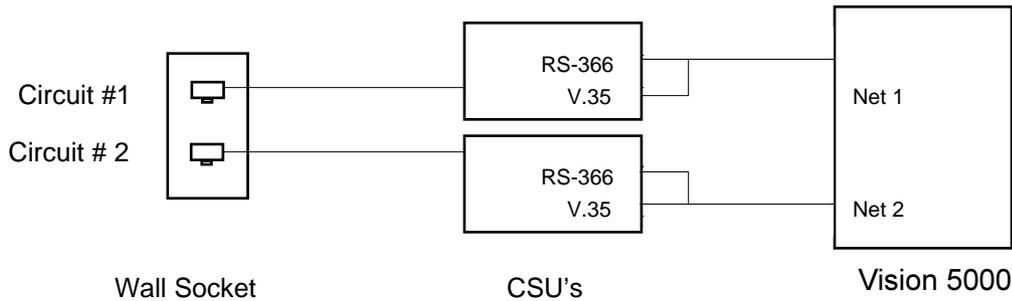
The cable set consists of a pair of RS-366/V.35 cables cable and should be connected thus:
