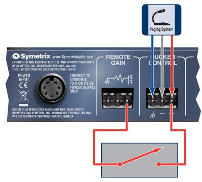
External switch or relay contact
