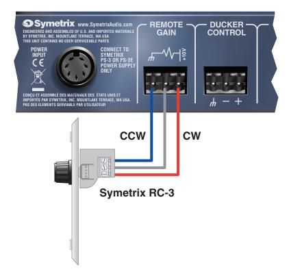
The **DUCKER CONTROL** input is normally connected to a line level audio signal from any source you would like to use to trigger a momentary decrease in volume (ducking).
