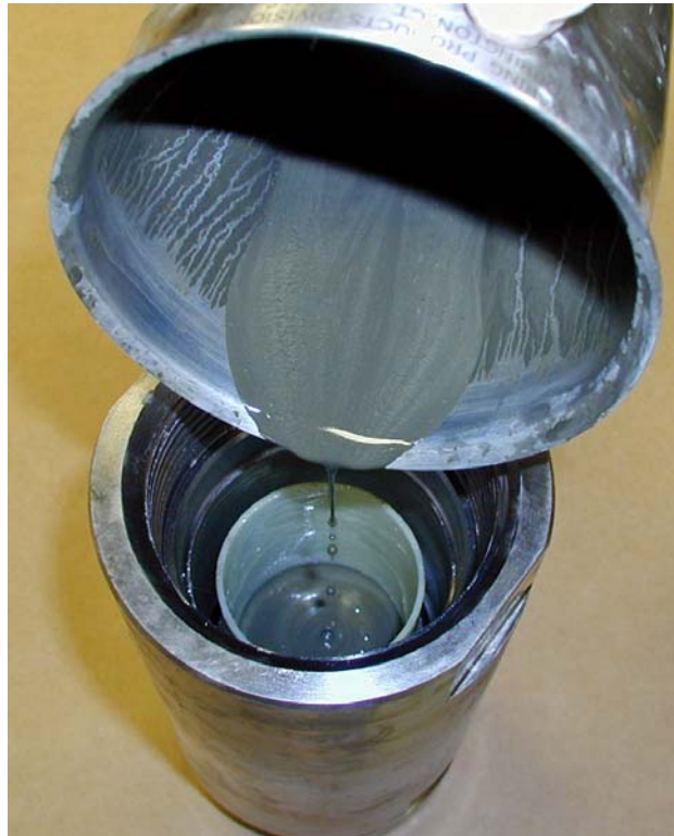
Figure 5-15 Pouring cement slurry into sample sleeve
