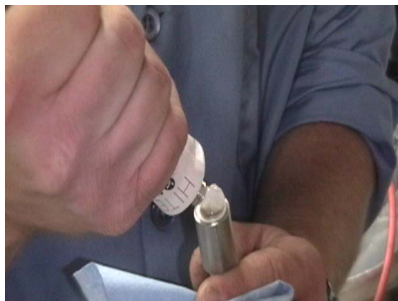
Figure 5-23 Coupling gel on transducer
