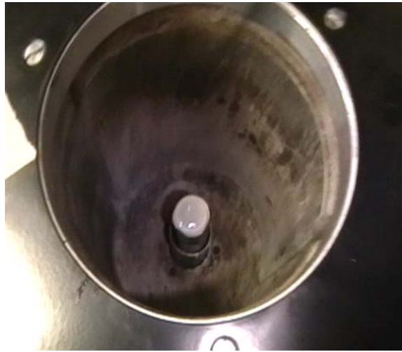
Figure 5-26 Bottom transducer in heating jacket
