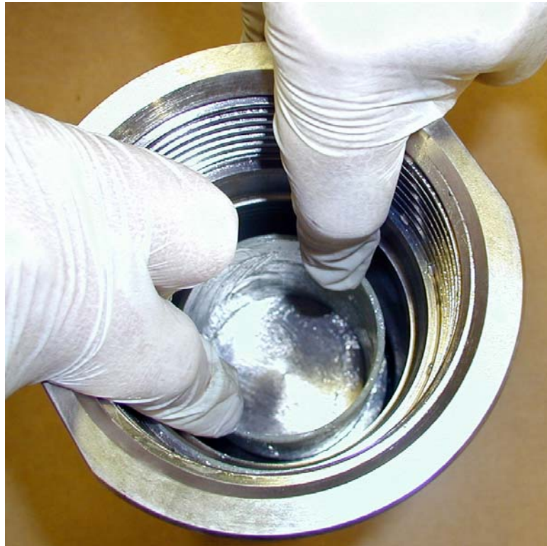
Figure 5-14 Seating sample sleeve into bottom lid groove
