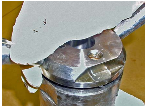
Figure 5-21 Water coming out of test chamber lid
