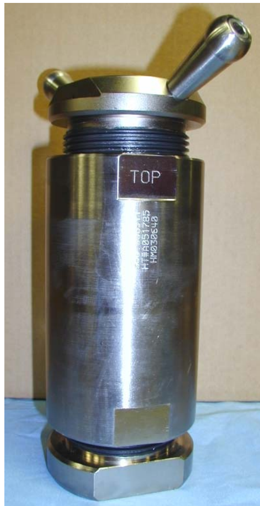
Figure 5-6 Chamber assembly with calibration rod
