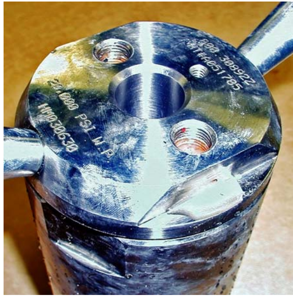
Figure 5-22 Top lid fully tightened
