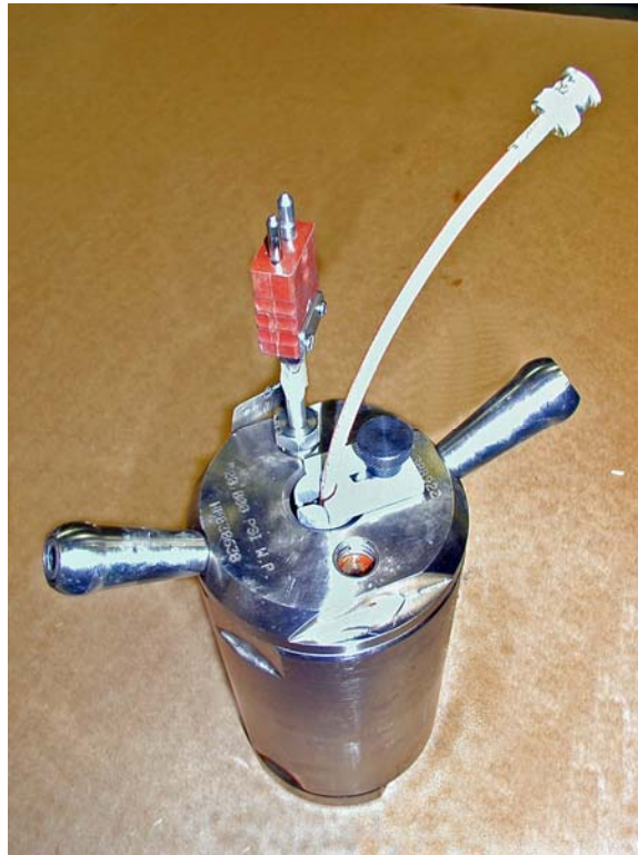
Figure 5-25 Assembled test chamber with thermocouple and transducer
