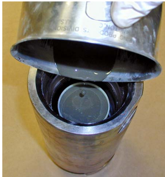
Figure 5-16 Fill the sample sleeve to the top
