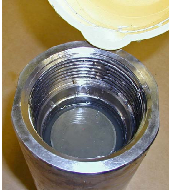
Figure 5-17 Pouring water around sample sleeve
