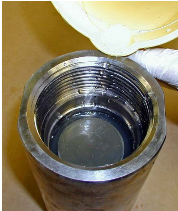
Figure 5-18 Water just covers the cement slurry
