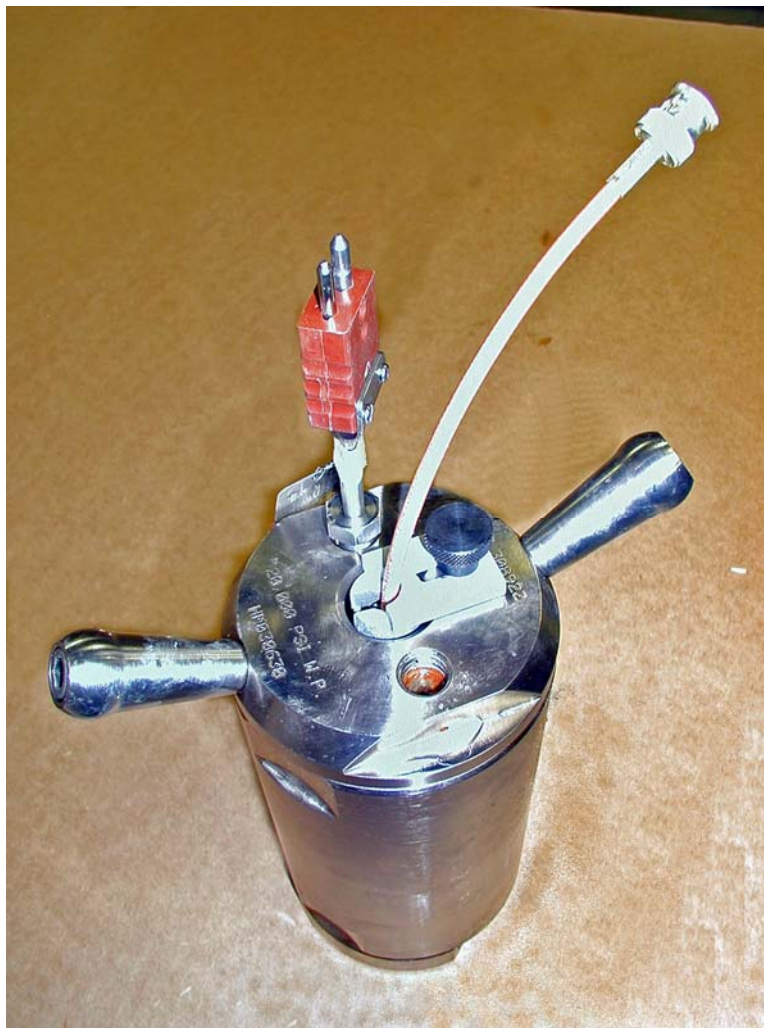
Figure 5-7 Assembled test chamber with thermocouple and transducer
