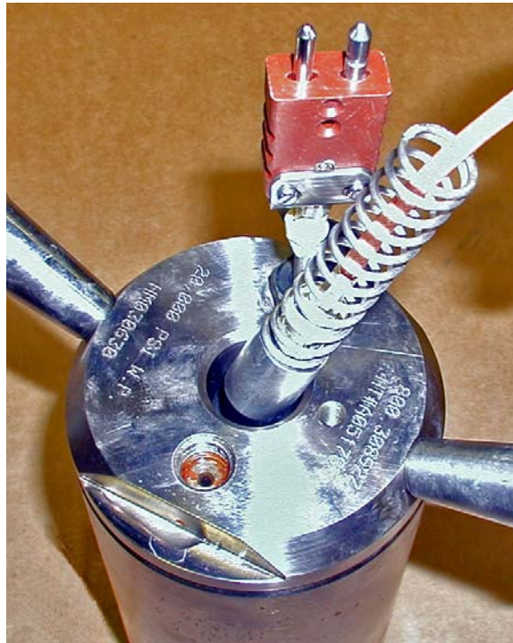
Figure 5-24 Inserting the transducer into the top lid
