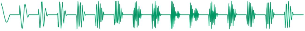
This waveform family simulates the sound of a trapezoidal pulse wave processed by a low-pass, peaking, band-pass, or high-pass resonant filter. The parameter controls the cutoff frequency of the filter. **pkzpulse** is particularly good at recreating the dirty, saturated sound, of a sawtooth filtered by the least academic of the 2-pole analog filters
