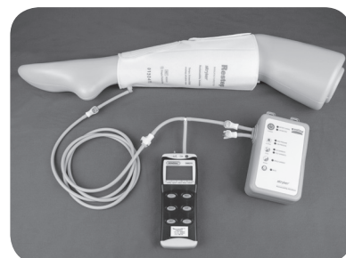
Attach garment, 6' tube, modified tube set, manometer, and pump.
