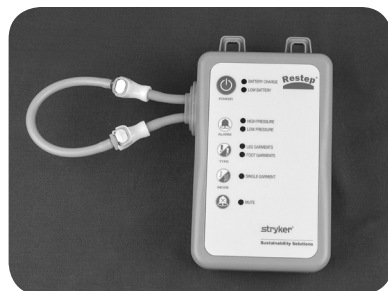
Attach male-to-male connector to outlet ports of pump.
