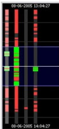
Timeline browser; displaying timelines for a camera layout with four cameras
