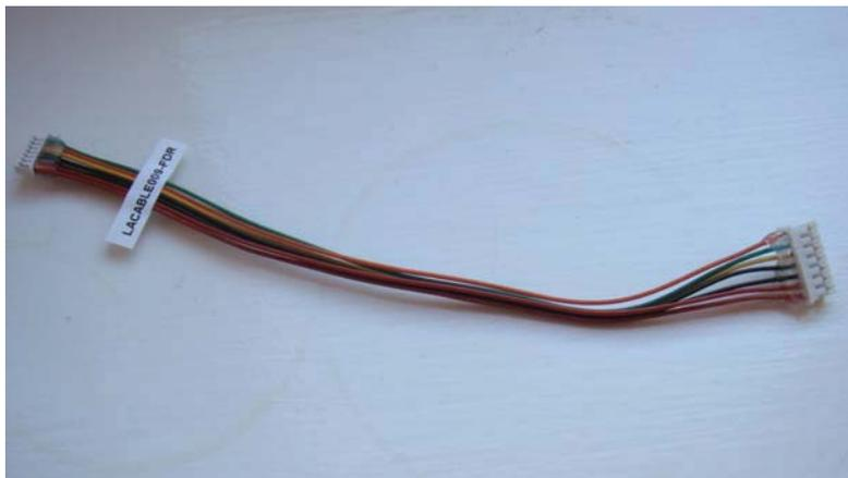
**Fig 2.9 Graphic Testing Board to Smart Touch Module cable**
