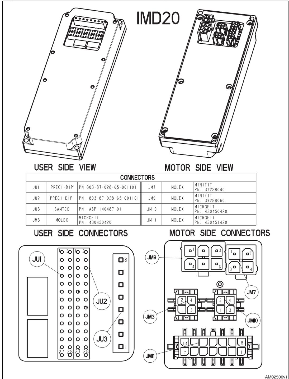
Figure 6. Mechanical data (dimensions in mm) continued
