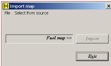
Submenu 'Import Map' – This is only used in off-line mode. This will enable the user to import a fuel, timing or pwm maps into the current map the user is working on. First you select the file which to import from and then under 'select from source' you can select which maps you want to import.
