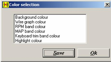
Submenu 'Color Selection' – This is used to change the color on the interface screen for the center viewing graph, and the marker cells of the map grid. Defaults that are 'saved' will be loaded every time the PC software is started.
