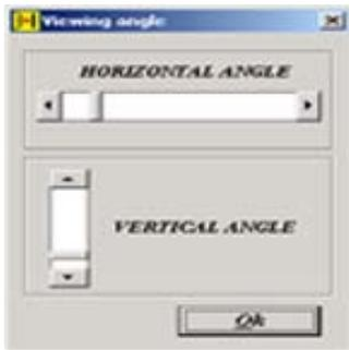
Submenu 'Angle' - This enables the user to rotate the 3D map. Viewing angle changes apply only to the Fuel, Fuel anti-lag trim, Fuel auxiliary trim, Spark, Spark anti-lag trim, Spark auxiliary trim, Spark back up and AFR target maps only.
