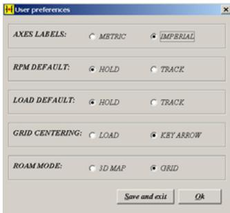
Submenu 'Preferences' – This is used to determine how you want the program to startup. Defaults that are 'saved' will be loaded every time the PC software is started.
