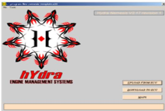
At the bottom right hand corner of the screen, there should be three selection tabs; Upload from ECU, Download to ECU, Maps.
