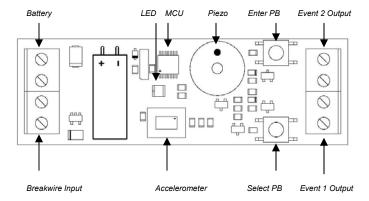
All user input and output connections are made to the compression terminals as shown. These terminals include: *Battery* (logic and/or pyro power), *Breakwire* (for a N/C wire loop switch), and *Event1/Event2* (for external pyro events or controls). All terminals are marked on the board silkscreen for reference.
