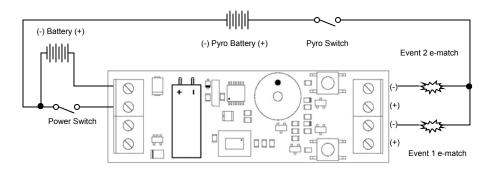
The unit has silkscreen labeling showing the designation of all the terminals and the associated polarity for each terminal where applicable. Stranded 20-22 AWG wire is recommended for the battery and power switch terminals.
