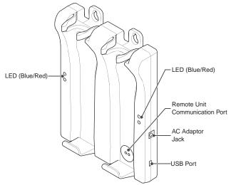
Before placing the RTR-601 into the dock, make sure that RTR-601 is not greasy or dirty as the dock is not waterproof and cannot be washed.
