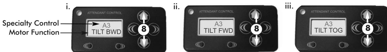
Images **i - iii** illustrate the program options available to assign the Tilt function to the A3 control/position.
