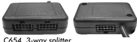
The **C654** splitter may be configured for use with up to three 4-Way Switches (one in each port), or it may be configured to utilize any switch combinations up to the maximum 12 switches.
