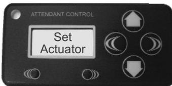
**Restricted Access:** Set Actuator functions are factory preset and password protected. Actuator functions may be individually programmed (i.e.; turned on and off). Please contact our Technical Service Department if any changes to the existing set-up are required.
