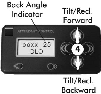
3. Press the **Up/Down** arrows (4) to adjust the seating system to the desired angle\*. (See **Recommended Tippy Angles** (p. 11)).
