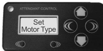
**Restricted Access:** Motor Type settings are factory preset and password protected. If any changes are required, please contact our Technical Service Department for authorization to reconfigure the existing Motor Type settings.
