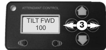
3. Use the **Up/Down** arrows to adjust the motor speed for the selected motor function:
