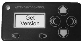
In order for our Technical Service Department to properly diagnose any potential issues, it may be necessary to identify the software version of the remote attendant control. Access to the Get Version display is available in the restricted program access section.
