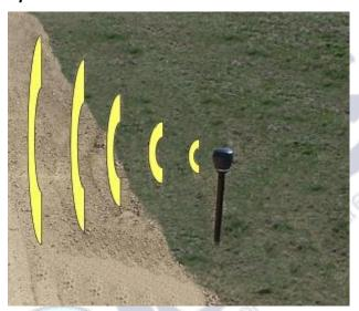
These sensors are used to recognize Arriving or Departing Vehicles from the Weighbridge. System can manage their signals to as to determine the traffic in/ out the weighbridge.
