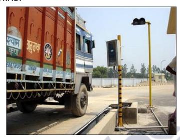
After Sensors send a call to IOBridge.Net, system will activate the RFID Read, so as to get the Vehicle ID & load all necessary info about the Vehicle.
