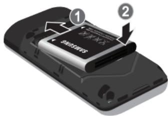
3. With the battery in position in the phone, align the back cover on the phone (1) and press down (2) until the cover clicks into place.
