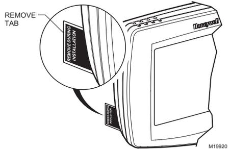
Fig. 23. Remove tab labeled REMOVE from thermostat back.
