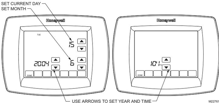
Fig. 24. Setting calendar and time after initial powerup.
