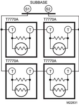
Fig. 18. Wiring four T7770A1006 (20K ohm) Sensors.
