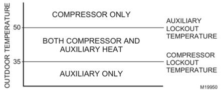
Fig. 27. Heat Pump Operation with Lockout Temperatures Set.
